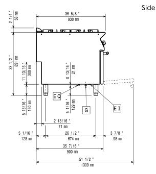
Electrical inlet (power) Gas connection
